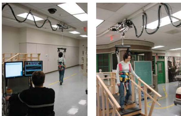
Fig 4. ZeroG dynamic over-ground body-weight support system.
