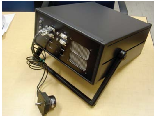
Figure 2: Controller for USM (MSUMC02: Mizoue project Japan Corp.)
