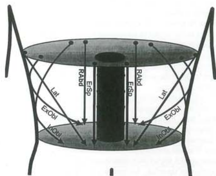
Figure 1. Schematic representation of trunk mechanics and muscle vectors used by model.
