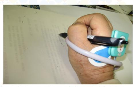
Fig. 1. Palm supporter and Sensor (Acceleration) are stuck on back of hand
